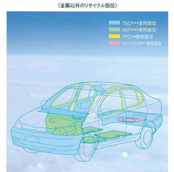
*4.TSOP: Toyota Super Olefin Polymer *5.RSPP: Recycled Sound-Proof Products *6.TPO: Thermo Plastic Olefin *7.リサイクルPP: Recycled Polypropylene
