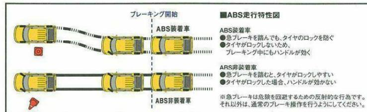
■EBD付ABS ※EBD[電子制動力配分制御]:Electronic Brake force Distribution
